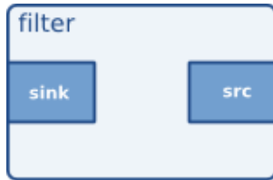
Figure 5-2. Visualisation of a filter element
