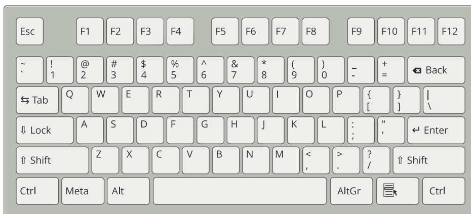
FIGURE 30.2: US KEYBOARD LAYOUT
