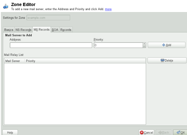
Figure 23.6 DNS Server: Zone Editor (MX Records)
